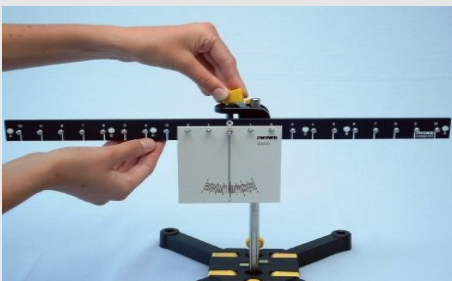
Fastening the double socket to the stand rod
